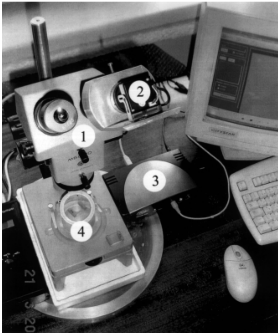
Fig. 1. Computerized system for estimating the microbial locomotion parameters: (1) microscope, (2) modular video camera, (3) digitizing unit, (4) set of Helmholtz coils.
